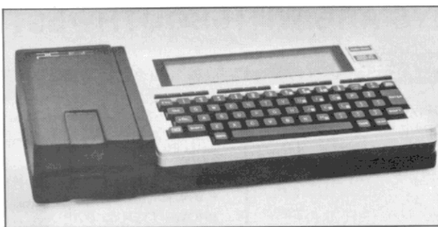
The PICDisk micro disk system includes CP/M 2.2 and T/Maker integrated software.
