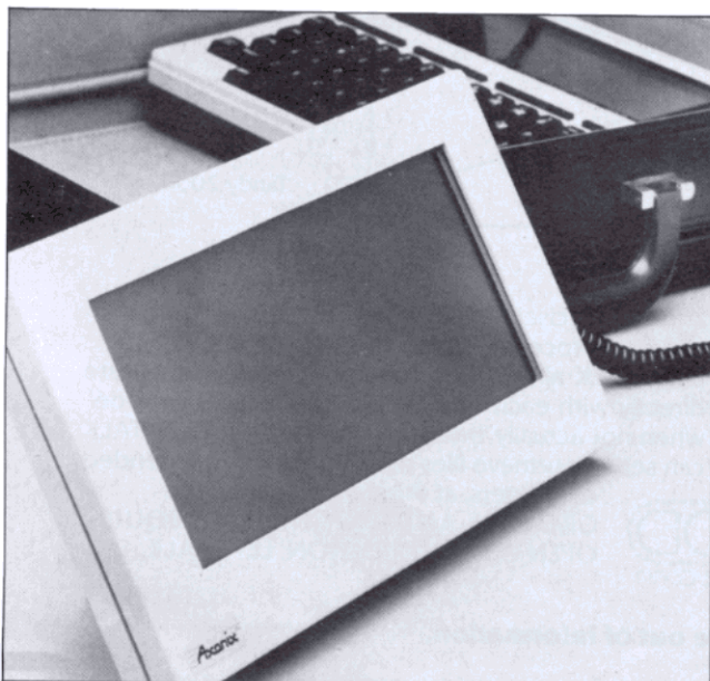
Thinview adds a 25-line LCD screen to the Model 100.
